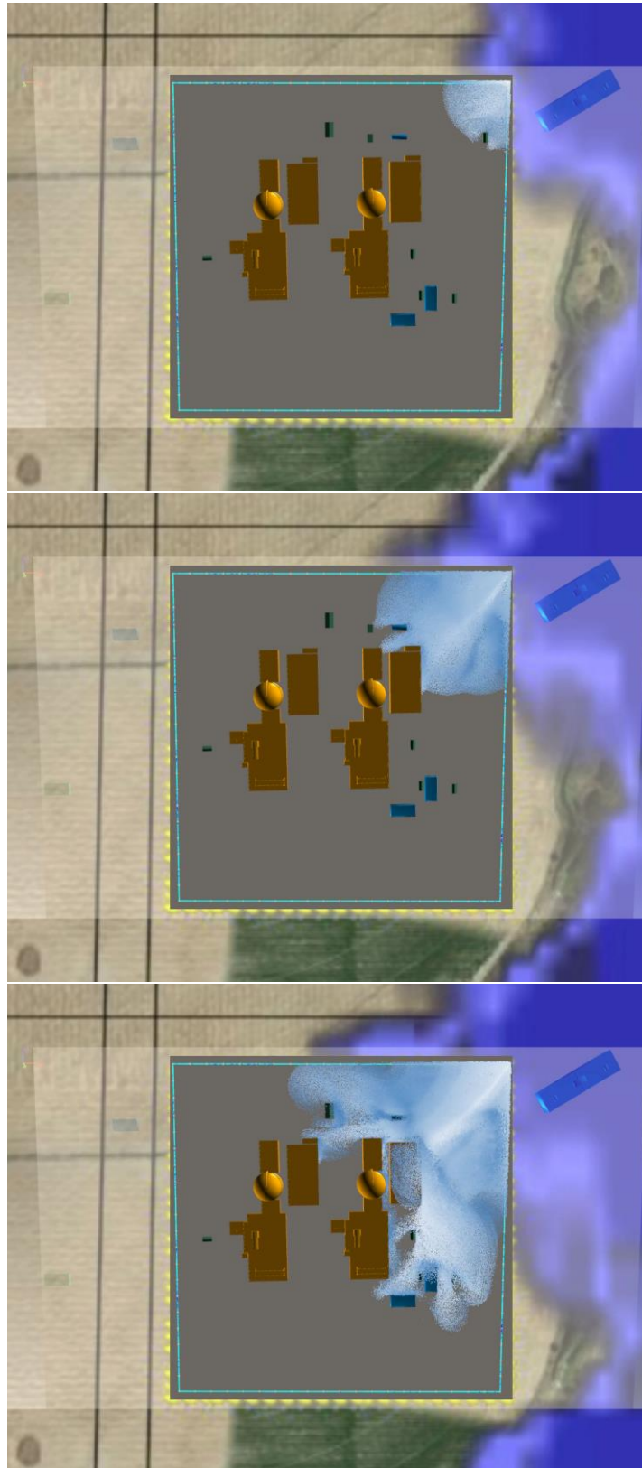
Figure 5: Flooding simulation output at the fictitious NPP site for both Neutrino IISPH (inner domain) and GeoClaw (outer domain) simulations at three different times: approximately 5 s (top), 15 s (middle), and 25 s (bottom) after the start of the inflow to the 3D domain. The coupling boundary is a square represented in cyan. The fluid particles in the inner domain are color-coded according to their speed, from dark blue (zero speed) to white (maximum speed).
