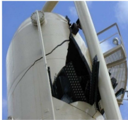
Figure 1 – Example of brittle fracture of a pressure vessel due to a crack [2].
